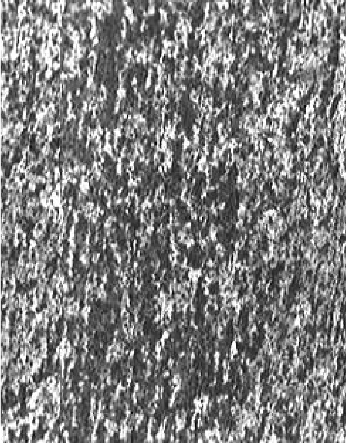
40 mm to surface (center) microstructure of SANGS™ AA 6061 as-formed bar of diameter 3-1/2" (above center-line, longitudinal view, X200)
